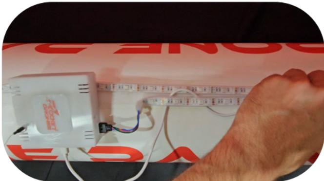
There is an arrow indicator on the tip of the RGB connector and on the timer case RGB plug. Align the arrows on the RGBs and the timer case. Ensure timer is placed in the center bottom of the gate. The timer will flash red until its connected to the USB dongle.
